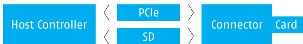
Figure 8: PCIe / SD support – most flexible solution – any card/ interface can be used
