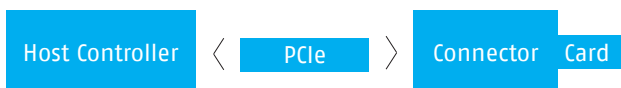
Figure 10: Native connection – PCIe-only support – not recommended because there is a SD card slot but SD cards are not recognized
