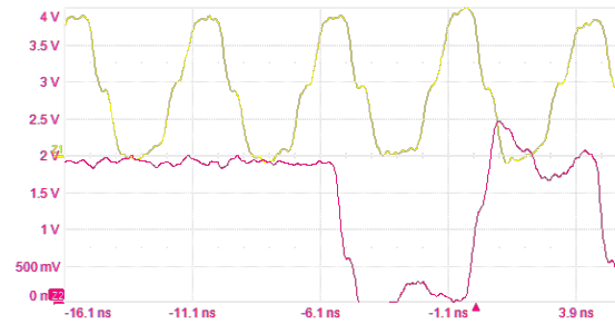
Figure 1: e.MMC interface at 1.8 V and 200 MHz (yellow: CLK, red: DAT0) with clear reflections on DAT0. However, it is not possible to determine whether these overshoots and undershoots also occur at the input stage.
