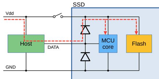
Figure 1: Drive powered via ESD diodes
