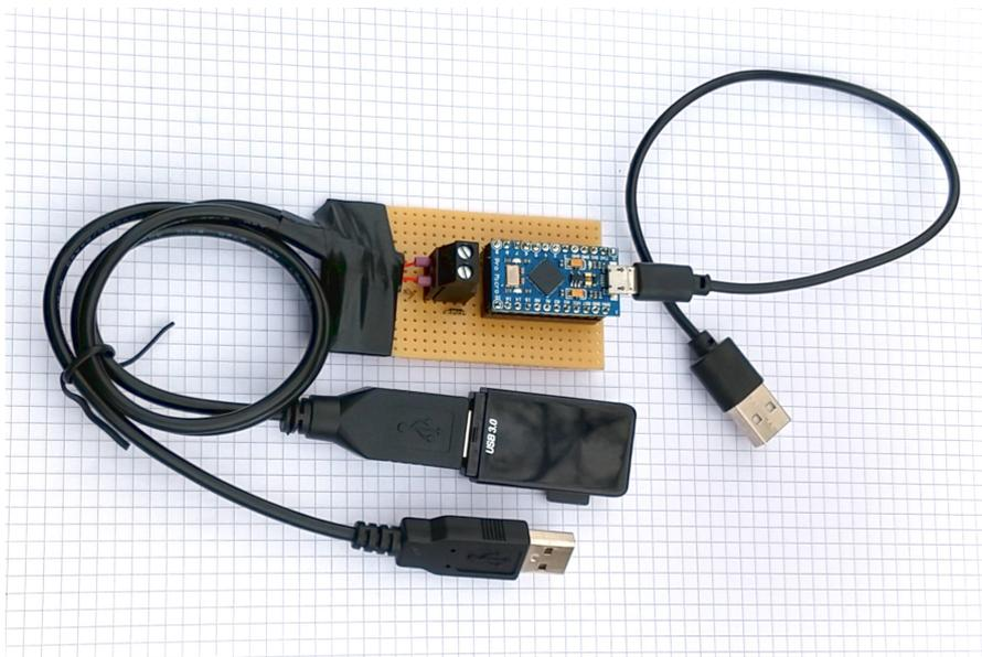
Figure 3: Setup with (micro)SD Card Reader
