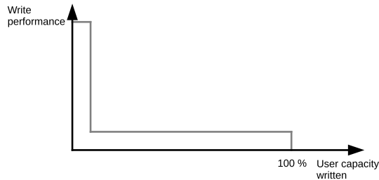
Figure 2: Sequential-Write with pSLC-Cache
