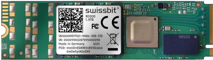
Figure 6: N3000 M.2 top view
